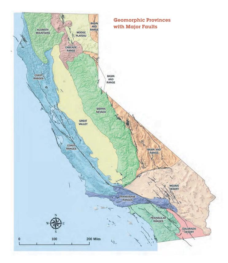
Figure 2-1: Geomorphic provinces with major active faults in black. Note how the faults virtually define many province boundaries.
