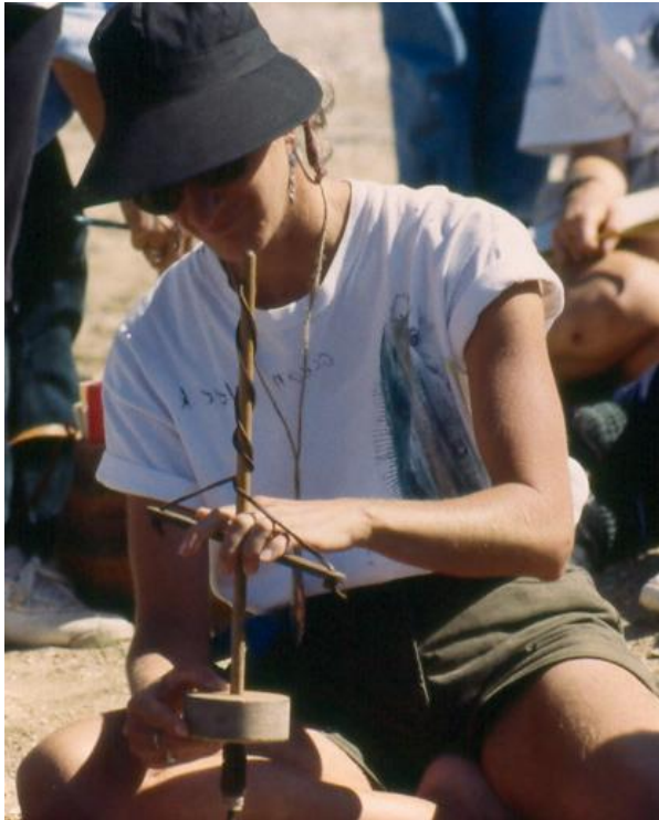
Teacher with a completed pump drill
