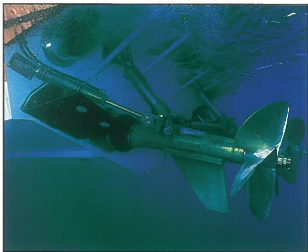
The Arneson Drive is a high-performance system designed to reduce drag while enhancing positive-thrust steering. It uses surface-piercing propellers.
