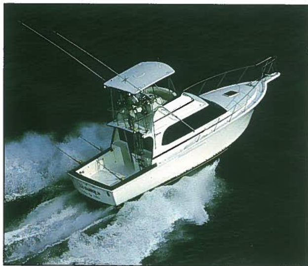
This sport-fishing boat with its planing-type hull has only part of the hull in contact with the water when on a plane.
