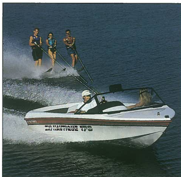
Having the tow line well forward of the transom will permit good maneuverability when towing a skier.
