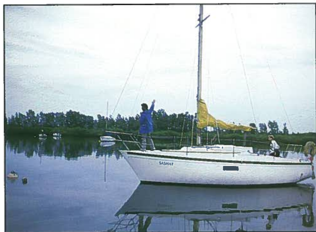
When picking up a mooring, approach slowly so that you come to a halt as you reach the buoy. The forward crew member should not have to hold the boat against the wind while picking up the pennant.
