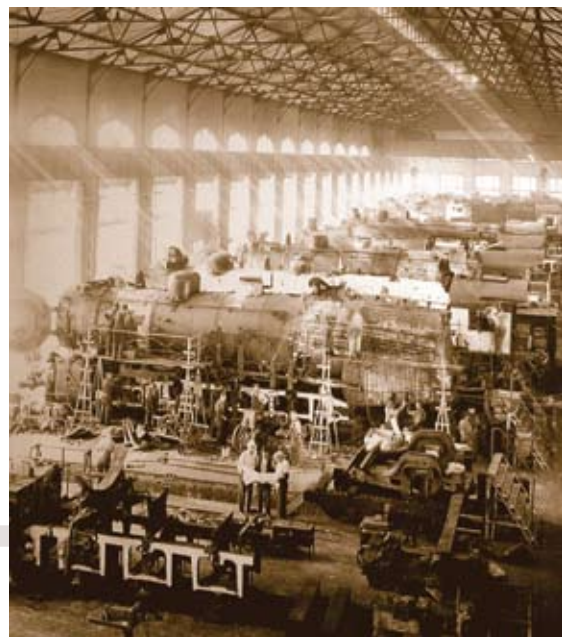
Steam locomotives are reassembled in the Erecting Shop following major overhaul.
