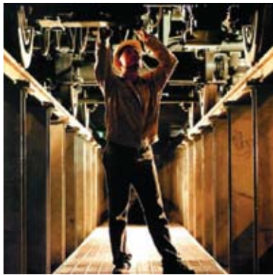
Wheels, axles and brakes being inspected
